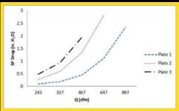
Figure 3: Static pressure drop across all plates at varying airflow rates relative to conical hood Velocity contours between plates show a higher capture velocity near the hood with diminishing improvement further upstream.
