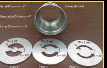
Figure 1: Design plates and the conical hood
