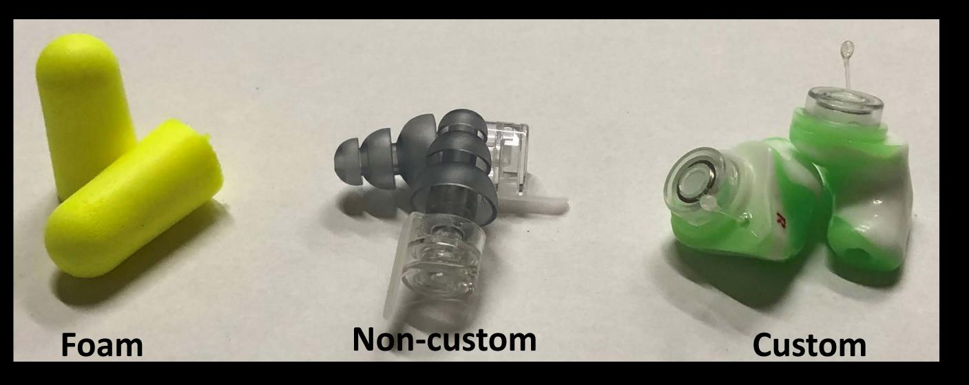
Figure 1. Illustration of HPD tested in this study
