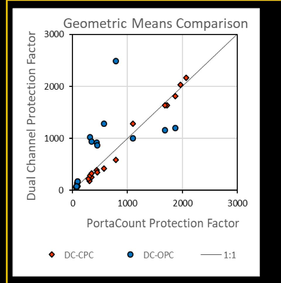
Overall geometric mean protection factor measured with the dual channel instruments relative to that measured with the PortaCount
