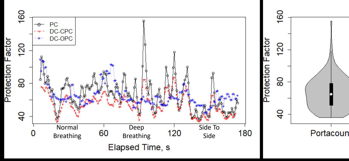
For this low target protection factor (PF=75), both dual-channel instrument measurements are relatively consistent with the PortaCount.
