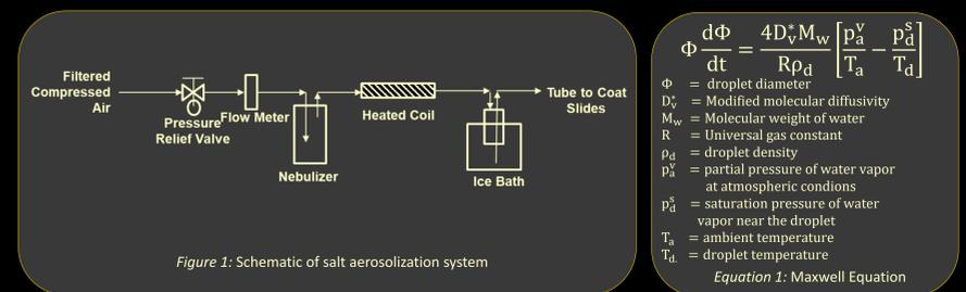
$$\Phi \frac{d\Phi}{dt} = \frac{4D_v^* M_w}{R\rho_d} \left[ \frac{p_a^v}{T_a} - \frac{p_d^s}{T_d} \right]$$
